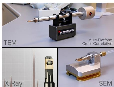
Along with the SEM system, our bulk liquid electrochemistry specimen holder is also available for transmission electron microscopy (TEM), and X-ray microscopy (XRM). The in-situ characterization made possible from the multi-modal platform provides complementary datasets suitable for accurate and reliable electroanalytical measurements of the sample at various length scales, and with complementary imaging and spectroscopy techniques.
