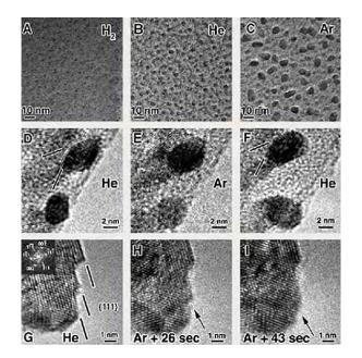
(**A** to **C**) Size evolution of Fe catalysts after 60 min under H2 (A), He (B), and Ar (C) at 500°C and 500 mtorr.
