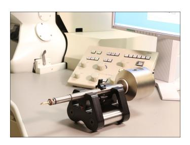
Hummingbird Scientific's Cryo-Biasing TEM Sample Holder enables researchers to conduct in-situ electrical biasing experiments of materials at cryogenic temperatures. The sample can be cooled down to liquid nitrogen temperatures with closed-loop control and accurate sensing of temperatures at the desired setpoint. Key characteristics of the holder include:
