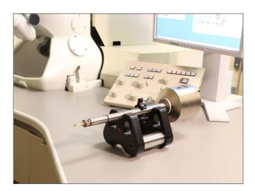
Hummingbird Scientific's Air-Free Transfer TEM Sample Holders enable the transfer of air-sensitive samples from the preparation chamber to the TEM inside the holder, either in high vacuum or in inert gas conditions. Example applications of this holder are in-situ materials experiments with air sensitive materials for:
