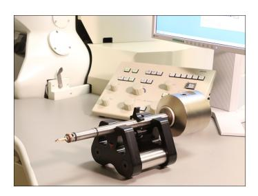
Hummingbird Scientific's Cryo-Biasing TEM Sample Holder enables researchers to conduct in-situ electrical biasing experiments of materials at cryogenic temperatures. The sample can be cooled down to liquid nitrogen temperatures and heated up to 1000°C with closed-loop control and accurate sensing of temperatures at the desired setpoint. Key characteristics of the holder include:
